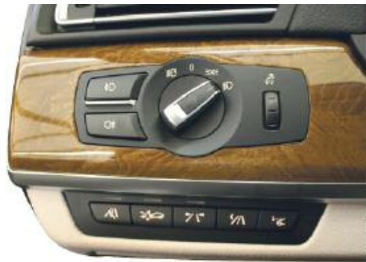
Light switch in position II
